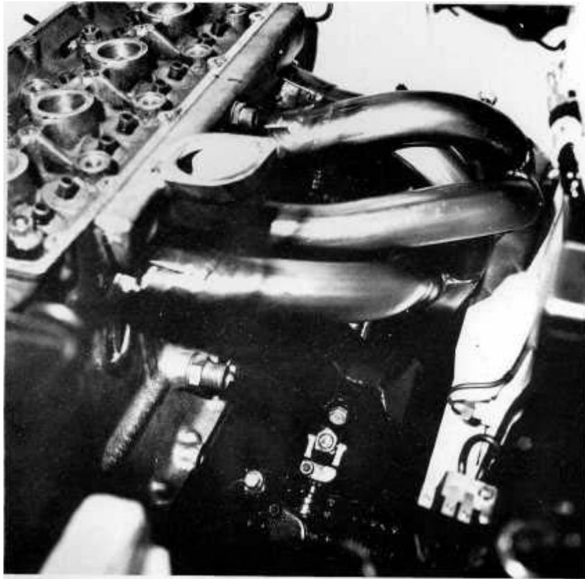
Tight exhaust manifold fit on I.h.d. car
